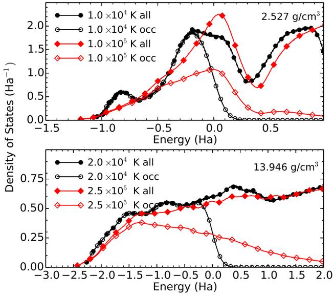
FIG. 10: Temperature dependence of the total (all) and occupied (occ) electronic DOS of dense, fluid nitrogen at densities of 2.53 and 13.95  $\text{g cm}^{-3}$ . Each DOS curve has had the relevant Fermi energy for each temperature subtracted from it.
