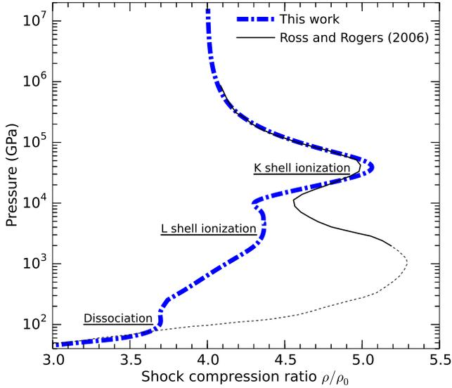
FIG. 13: Comparison of our combined PIMC and DFT-MD Hugoniot curve with predictions of ACTEX plasma model calculations by Ross and Rogers<sup>8</sup>. The dashed line portion of the plasma model curve indicates where the ACTEX results were interpolated to match experimental data below 100 GPa. The initial density was  $\rho_0 = 0.8076 \text{ g cm}^{-3}$  ( $V_0 = 28.80 \text{ \AA}^3/\text{atom}$ ).
