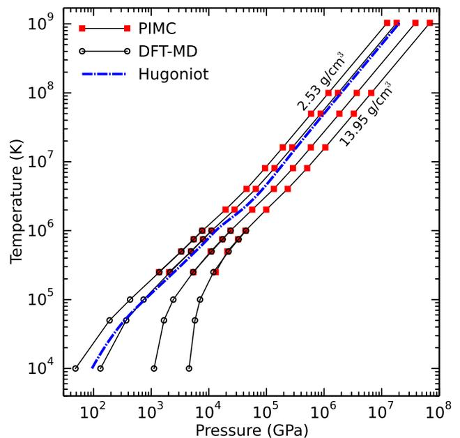
FIG. 2: Temperature-pressure isochores computed with DFT-MD (circles) and PIMC (squares) at densities of 2.5, 3.7, 7.8, and  $13.9 \text{ g cm}^{-3}$ . The blue dash-dotted line shows the Hugoniot curve for an initial density of  $\rho_0 = 1.035 \text{ g cm}^{-3}$
