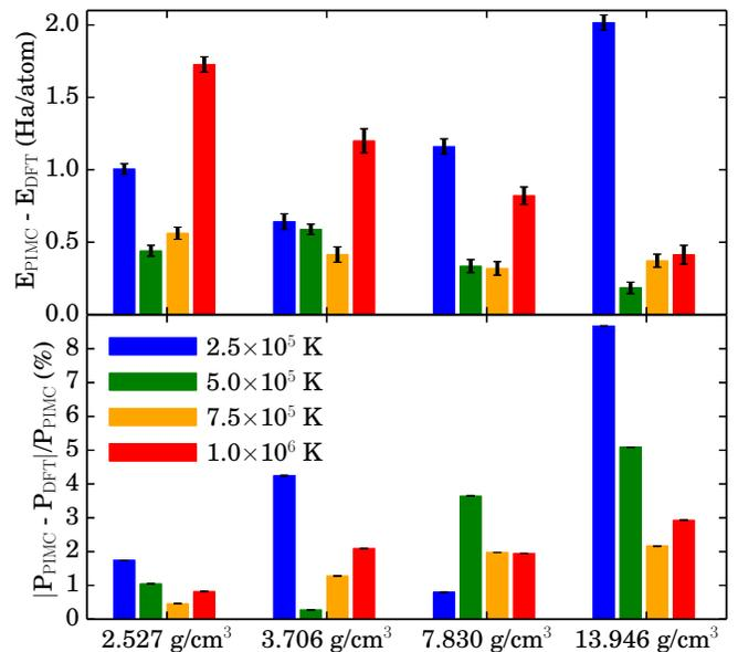
FIG. 4: Differences in PIMC and DFT-MD energies and pressures. The top panel shows energy differences, while the bottom panel shows the absolute relative error of pressure in percent. One- $\sigma$  errors in the differences are shown in black.
