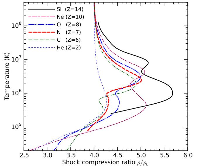
FIG. 15: Comparison of the shock Hugoniot curves for different materials. The initial volume  $V_0$  has been chosen such that the density of the electrons is the same for all materials ( $V/N_e = 3.586 \text{ \AA}^3$ ). The various maxima in compression corresponds to excitations of electrons in the first and second electron shells.
