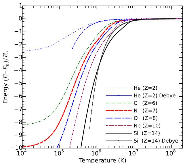
FIG. 17: Internal energy vs. temperature is shown for the isochores in Fig. 16. The energy contribution from a fully-ionized, non-interacting plasma,  $E_0$ , has been removed in order to compare only the interaction effects.
