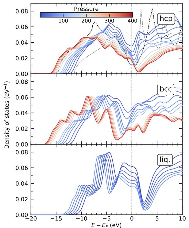
FIG. 13. Electronic density of states of Be at 3000 K. DOS of hcp Be at 0 and 200 GPa from Ref. [97] are shown in dot-dashed and dashed lines in the upper panel.
