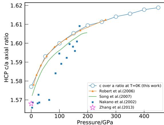
FIG. 6. Variation of the  $c/a$  ratio of hcp phase of beryllium with pressure. Open circle: DFT calculation in this work; Yellow triangle: first principle calculation by Robert *et al.* [16]. Green curve: classical analytic mean-field potential method by Song *et al.* [70]; Blue square: X-ray diffraction DAC experiment by Nakano *et al.* [24]; Magenta star: experimental value at  $P = 0$  GPa from Zhang *et al.* [71].
