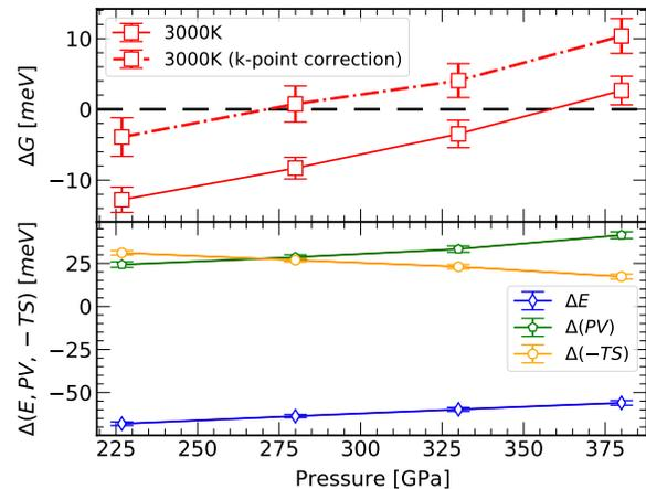
FIG. 3. Gibbs free energy difference,  $\Delta G \equiv G_{\text{hcp}} - G_{\text{bcc}}$ , between hcp and bcc phases along the  $T = 3000$  K isotherm. The different contributions to  $\Delta G = \Delta E + P\Delta V - T\Delta S$  are shown in the lower panel.
